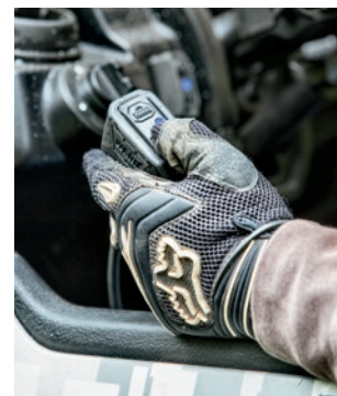
The color LED display on your hand-held or dash-mounted control switch delivers user feedback, including information on winch temperature and load
