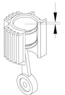
Deck height should measure between 0.50mm and 0.70mm [0.020 and 0.028"]
