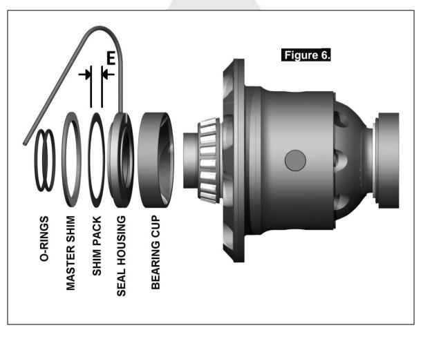
Make sure the grooves and airway of the seal housing are clean and free from any contaminants (e.g. water, dirt, metal filings, etc.).
