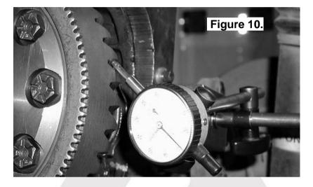
Refer to your vehicle service manual for the specified maximum and minimum amounts of backlash. If the backlash is not within the specifications then the differential will have to be removed and reshimmed.
