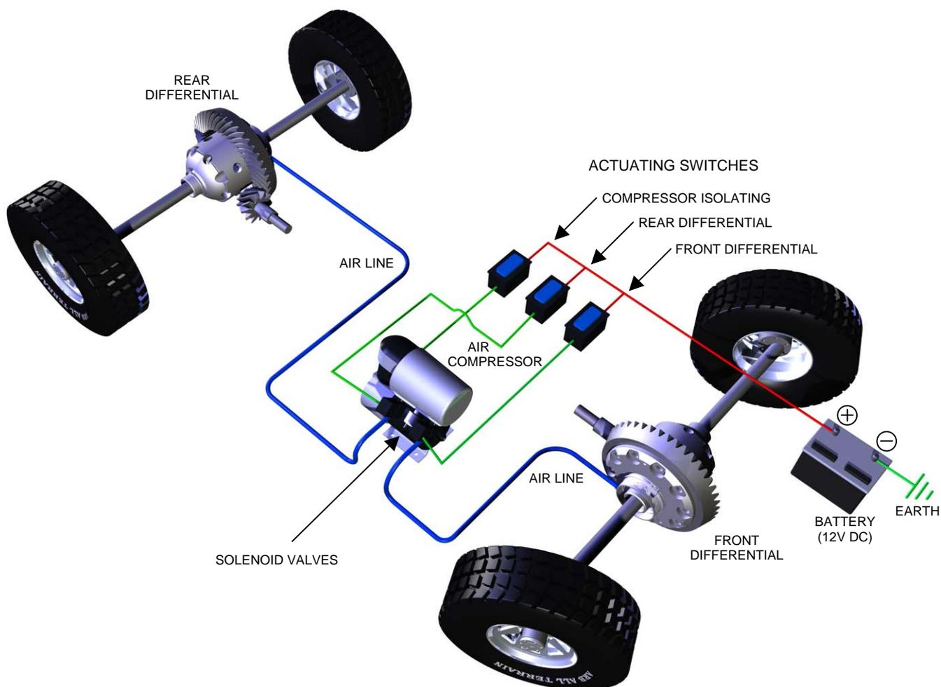
The air compressor is started with the air compressor switch, and a pressure switch maintains the air pressure in the reservoir between 585kPa [85psi] and 690kPa [100psi]. When the Air Locker switch is operated, the relevant pneumatic solenoid valve opens, allowing compressed air down the line to the differential.
