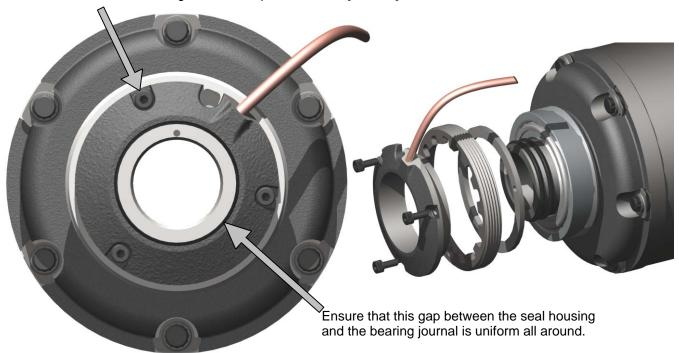
The following installation procedure is recommended to ensure that the seal housing is concentric to the bearing journal and that the seals are airtight:
